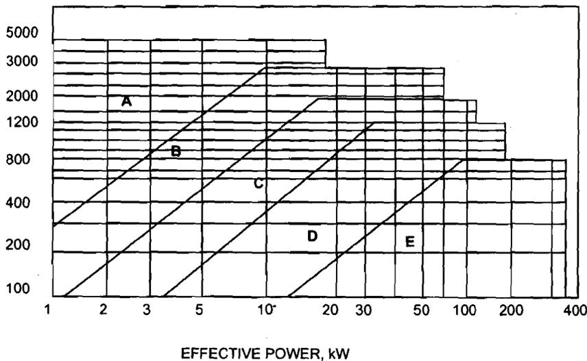
Figure 9.11 : Effective Power of Belts as Function of RPM of Small Shear (Based on Goodyear Hand Book)
