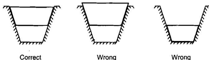
Figure 9.7 : Correct and Wrong Mountings of V-belt in Sheave
