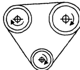
(g) Belt Drive with Several Pulleys Rotating in the Same Direction
