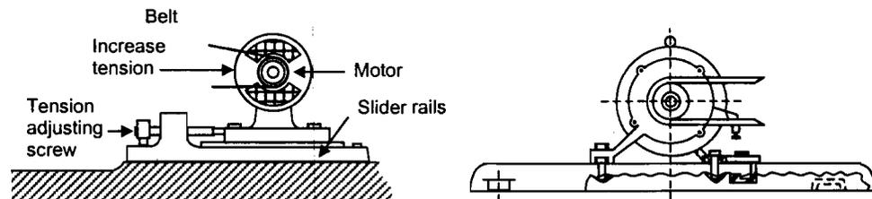
Figure 9.6 : Adjustable Motor Base to Help Adjust the Center Distance of the Belt Drive
