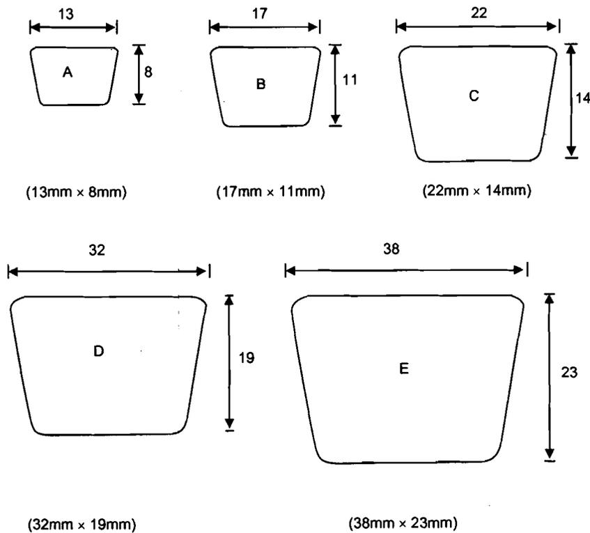
Figure 9.10 : Various V-belt Sections
