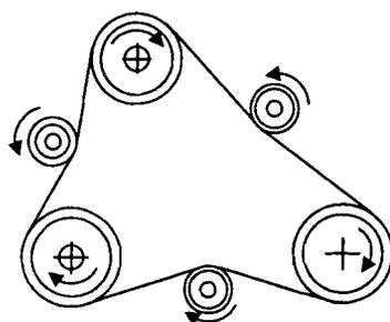
(h) Belt Drives with Several Pulleys Rotating in the Same and Opposite Direction
