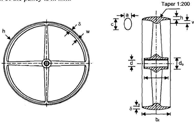
Figure 9.5 : A Pulley with Arms Connecting Hub and Rim
